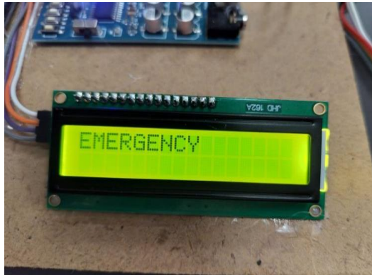
Fig. 5: LCD Output Display Showing Detected Gesture Message EMERGENCY
