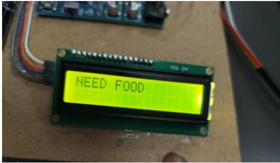
Fig. 4: LCD Display Showing Recognized Gesture Output NEED FOOD
